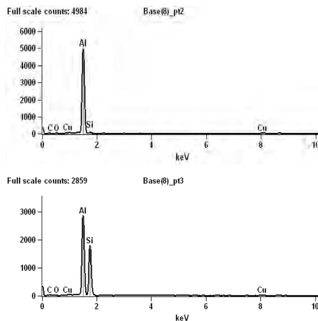
Fig. 5. Chemical composition of aluminium AlSi11 alloy (1) and inter-phase boundary (2)
