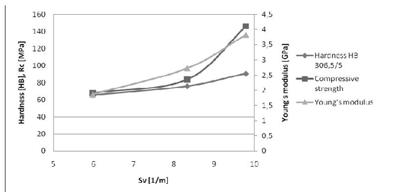
Fig. 7. Effect of specific surface fraction of interphase boundaries on mechanical properties of  $\text{Al}_2\text{O}_3/\text{AlSi11}$  composites
