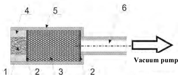
Fig. 1. Design of sampler used for subpressure infiltration of ceramic preforms: 1 - preform sample, 2 - mesh, 3 - filter (cooler), 4 - sample (preform) sealant, 5 - casing, 6 - vacuum pump connection
