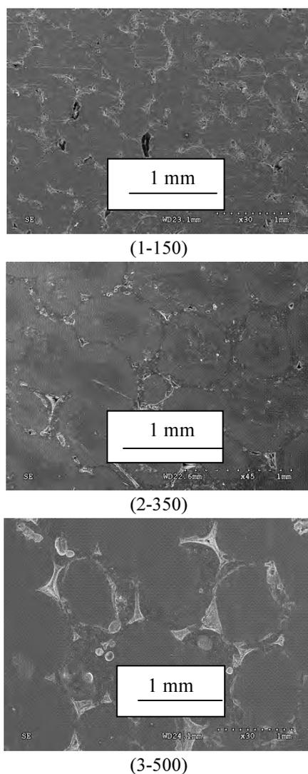
Fig. 4. Microstructure of  $\text{Al}_2\text{O}_3/\text{AlSi11}$  composites (samples 1 - 150, 2 - 350, 3 - 500, respectively)
