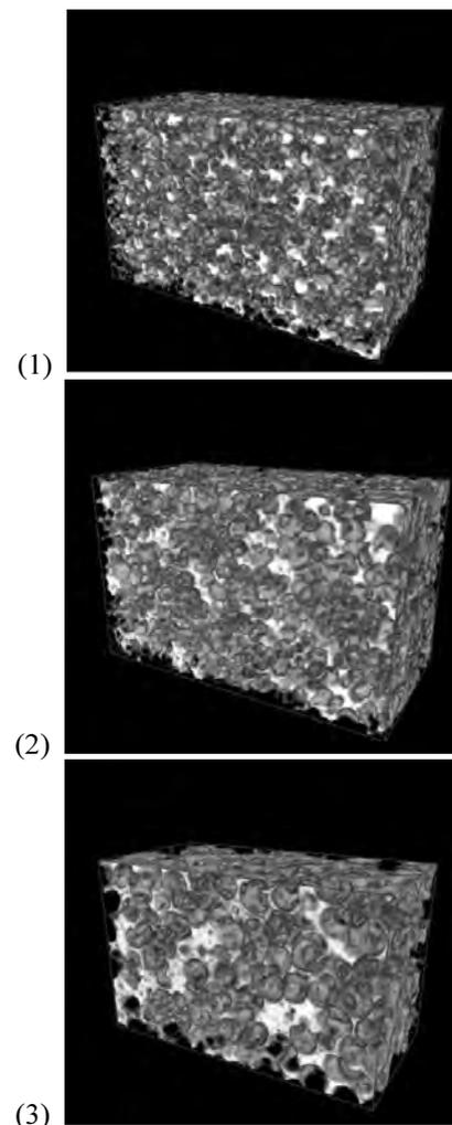
Fig. 3. X-ray tomography images of porous  $\text{Al}_2\text{O}_3$  ceramics (samples 1 - 150, 2 - 350, 3 - 500, respectively)
