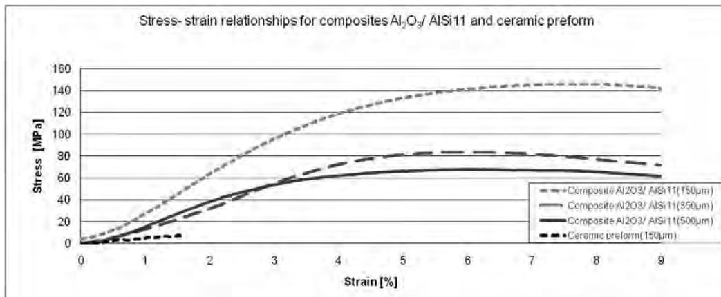
Fig. 6. Typical stress-strain curves for ceramic and  $\text{Al}_2\text{O}_3/\text{AlSi11}$  composites
