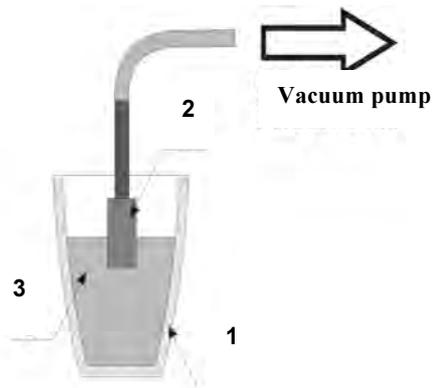
Fig. 2. Transportation by suction of liquid alloy to sampler containing ceramic preform: 1 - melting-pot, 2 - liquid alloy, 3 - sampler
