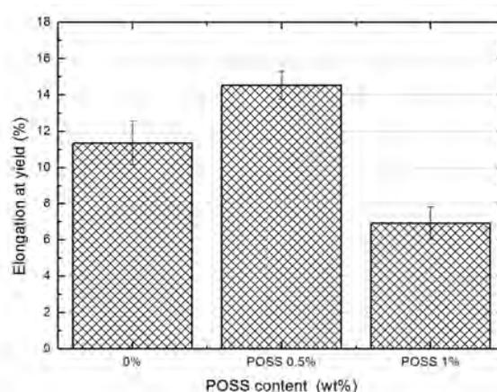
Fig. 5. Elongation at yield of neat POM and POM/POSS composites with different POSS content
