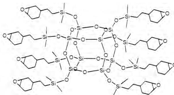
Fig. 2. Chemical structure of octakis (*dimethylsiloxy, ethyl epoxy-cyclohexy*) octasilsesquioxane (POSS)
