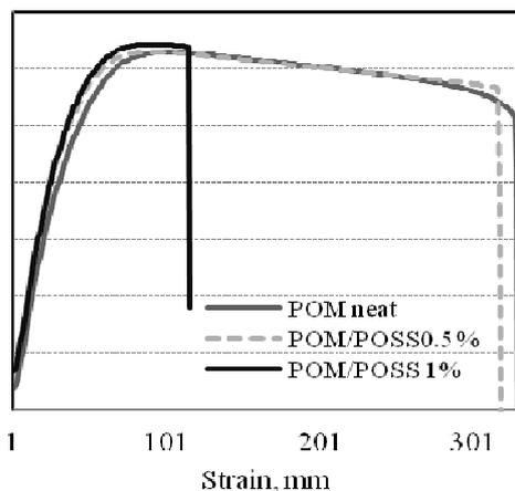
Fig. 3. Comparison of stress-strain curves of POM neat and POM/POSS composites with different POSS content
