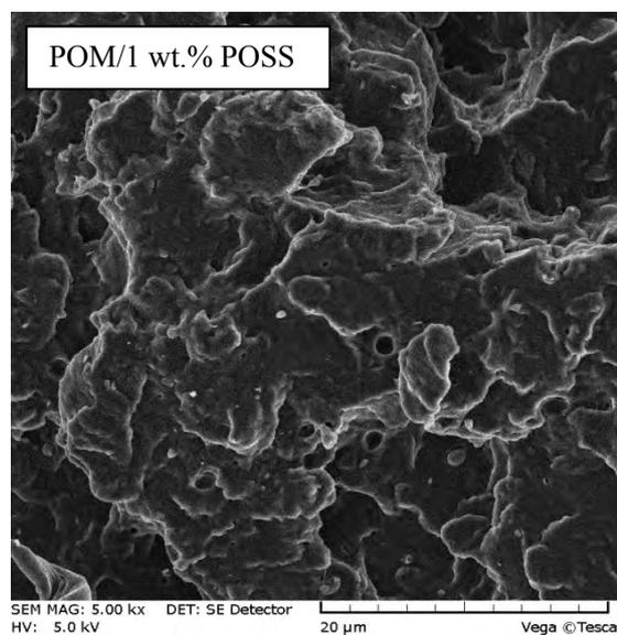
Fig. 9. SEM micrograph of POM/POSS composites with 1 wt.% POSS
