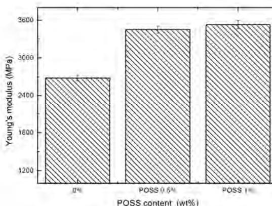
Fig. 6. Young's modulus of neat POM and POM/POSS composites with different POSS content
