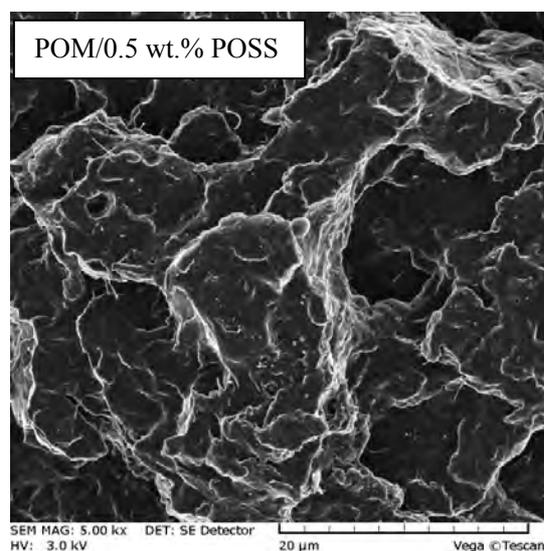
Fig. 8. SEM micrograph of POM/POSS composites with 0.5 wt.% POSS
