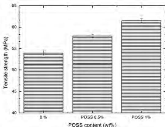
Fig. 4. Tensile strength of neat POM and POM/POSS composites with different POSS content
