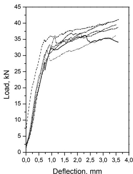
Fig. 8. Beams with smooth steel rods
