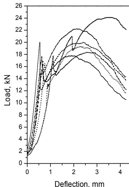
Fig. 6. Beams with polypropylene fibres
