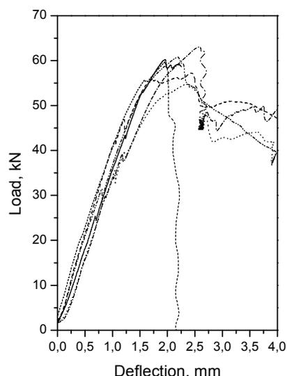
Fig. 9. Beams with ribbed steel rods
