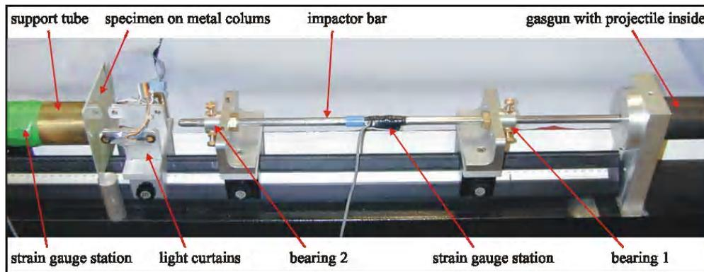
Fig. 2. Components of the Hopkinson device [6]
