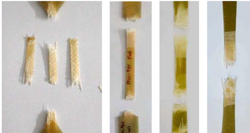
Fig. 3. Fracture types of high-speed test specimen with conventional and optimised geometries
