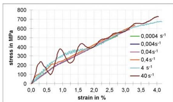
Fig. 4. Strain rate dependent stress-strain diagrams of glass fibre reinforced specimen
