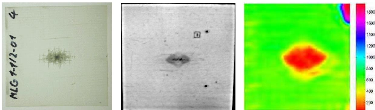
Fig. 7. Multi-layered knitted fabric test specimen after impact and associated optic excited thermography photo and ultrasonic inspection exposure
