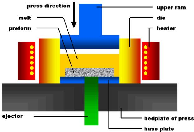
Fig. 1. Schematic sketch of a squeeze cast tool
