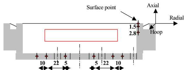
Fig. 2. Geometry of the brake drum - measuring points
