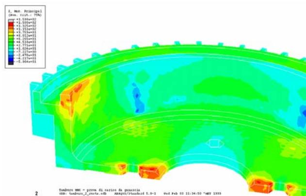
Fig. 4. Finite element calculation: Analysis of the maximum principal stresses
