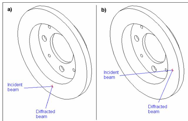
Fig. 3. Lay out of the X-ray diffraction measurement
