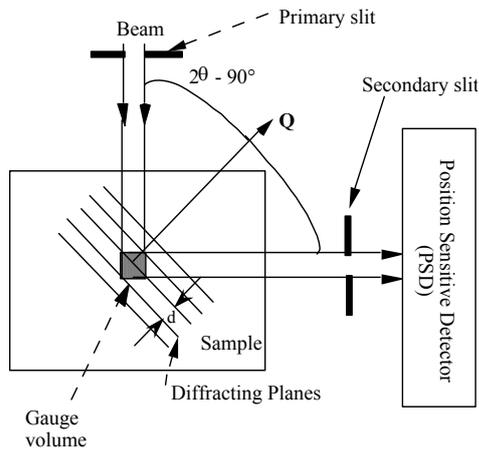
Fig. 1. Lay-out of a neutron diffraction experiment for residual stress measurements
