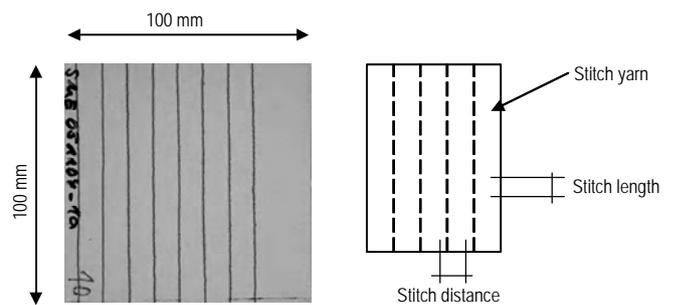
Fig. 4. Specimen configuration (stitch yarn: aramid, stitch length 4.8 st/10 mm, stitch distance 10 mm)
