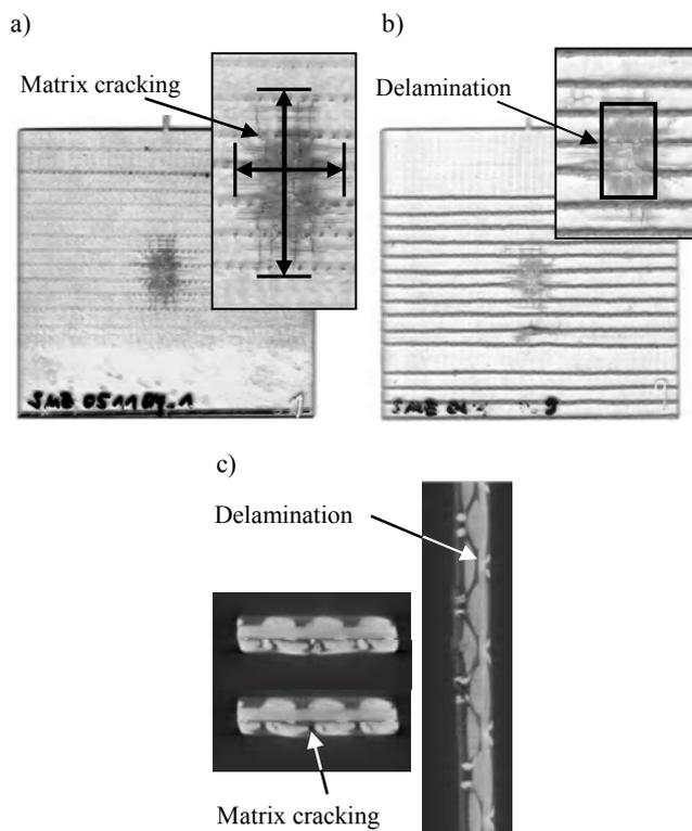
Fig. 7. Specimen damaged due to impact: a) glass stitching, b) aramid stitching, c) CT-scan [3]
