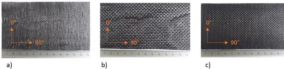
Fig. 1. Prepregs used in tests, a) UD 200g/m<sup>2</sup>, b) plain 160 g/m<sup>2</sup>, c) plain 204 g/m<sup>2</sup>
