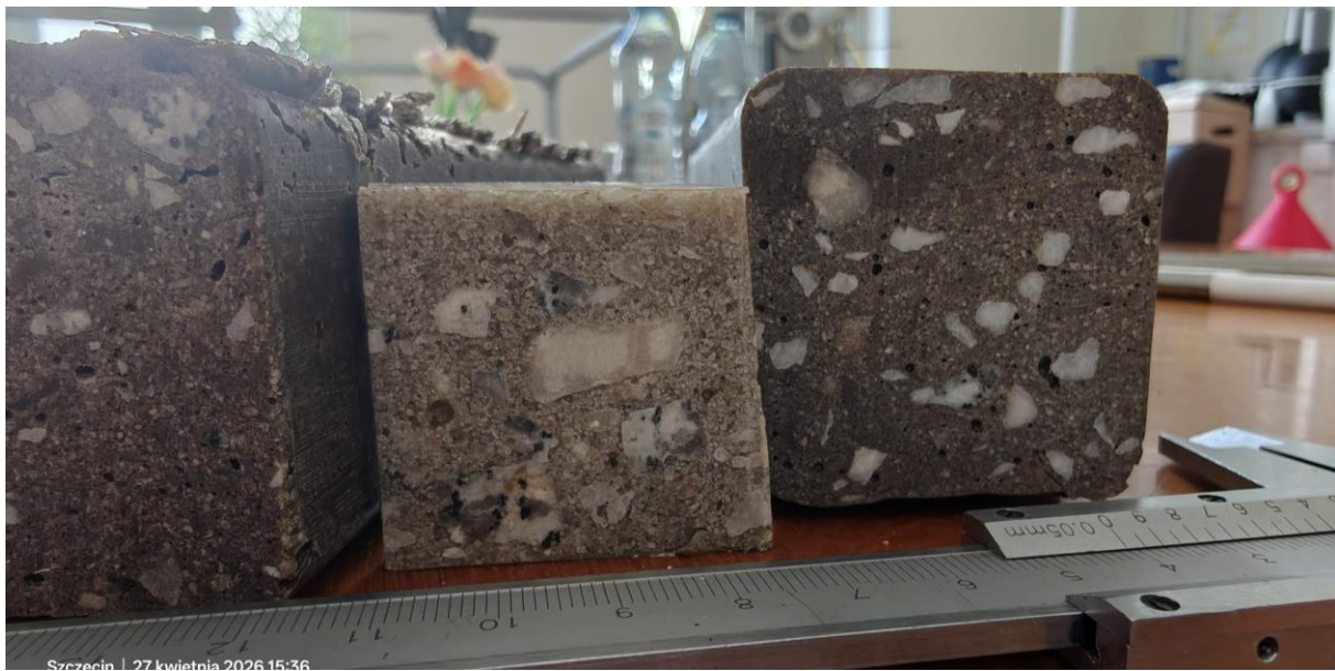
Fig. 2. View of manufactured polymer concretes
