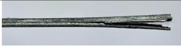
Figure 14. Crack front migration during test for specimen DCB-5.
