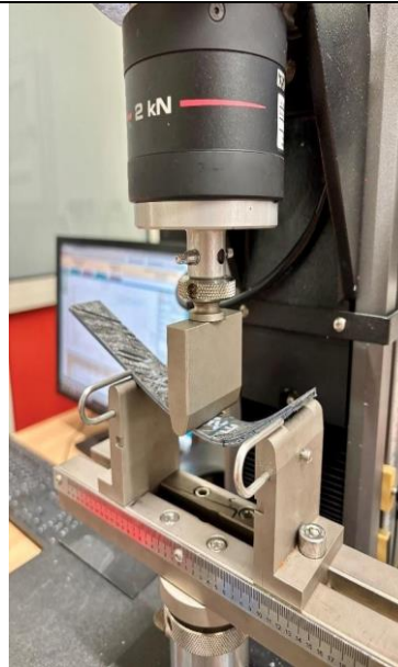
Figure 10. ENF test setup with specimen during loading.
