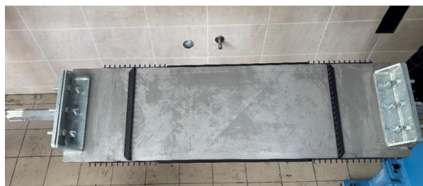
Figure 1. Rectangular plate prepared for filament winding.
