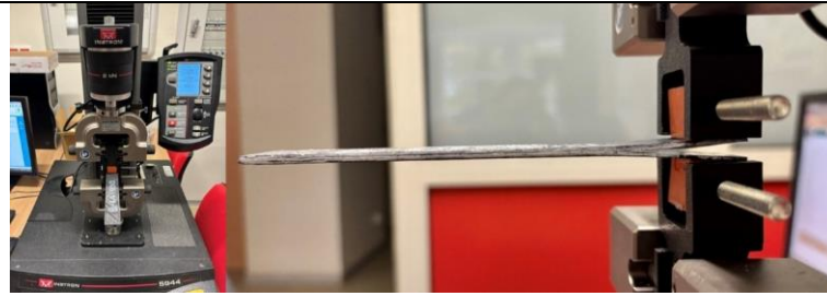
Figure 9. DCB specimen mounted in testing setup.
